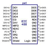
Ground pins are provided for each signal on the debug header, with extras at each side, so a single row connector could be used if preferred.
